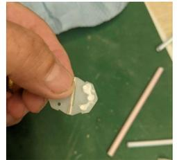
Now, you can insert the hinge into the slot and some glue will squeeze out. I usually use a damp paper towel to remove the excess glue. Once you have completed all the hinges, just leave it sit for about an hour and then come back to it and work the hinge surfaces. It may feel stiff at first but it will loosen up after a few flexings of the hinge.
