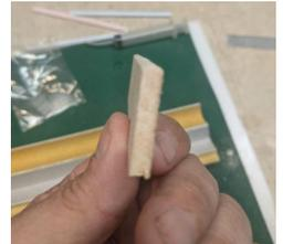
Once the slots are all cut in, I take a tool that I made to recess the slot on one surface to allow for the hinge center to get close to keep the gap at a minimum.
