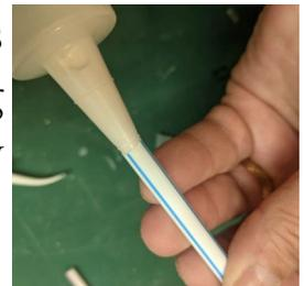
Next, pinch the end of the straw and insert it into the hinge slot about 1/8 of an inch. Next, squeeze the straw from the opposite end to push the glue into the slot until it starts to come out. Remove the straw and wipe away any excess glue. Now, repeat the glue on the hinge as in the picture above, and insert the hinge.
