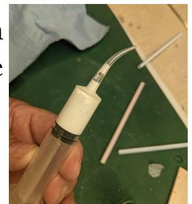
You then insert the tip of the syringe into the center of the slot and inject the glue until it comes out of the slot.
