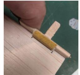
The next step is to glue in the hinge. This is where I have learned that the best glue to use for this is Zap Canopy Glue #560. This is white glue that is much thinner than the normal white glue but it is formulated to bond plastic to wood. Here is the glue and what you need. I use two methods for inserting the glue into the slots.
