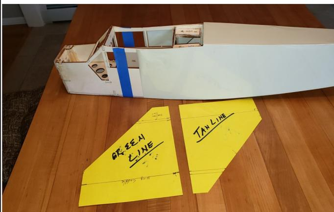
Since I was changing colors along the length of the fuselage, I measured and cut stencils (see picture) that allowed me to neatly overlap the material in a uniform manner. When applying UltraCote over UltraCote, eliminating bubbles is essential. I first moisten the base
