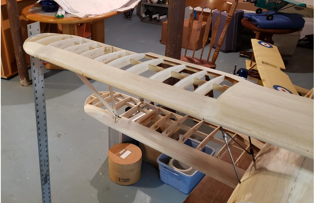
The plans call for simply screwing the top wing onto the cabanes. I am not sure how one would make all the adjustments when you do that, so I instead chose to solder lugs onto the cabanes and use 6-32 bolts attached to blind nuts embedded in the wing.
