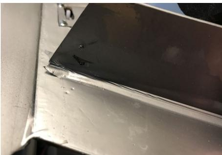
I installed the servos and the control horns on the wing. You must cut off the screws on the control horns so they don't interfere with the flaps retracting.
