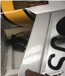
Then, I used Monokote to create a hinge for the flap onto the wing.
