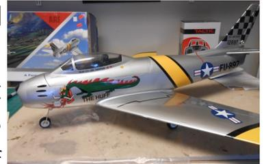
runway to take off, and it lands in excess of 50mph. Once airborne, the jet flies great. Yet, in order to correct the problem of the long takeoff and fast landing speed, I decided to add a set of split flaps to the model. I did not split the bottom of the wing, but rather just added them to the airfoil. They are 1/16" thick and laminated from 1/32" plywood. The epoxy lamination made them very strong, so I don't anticipate any problems. Let's begin.
