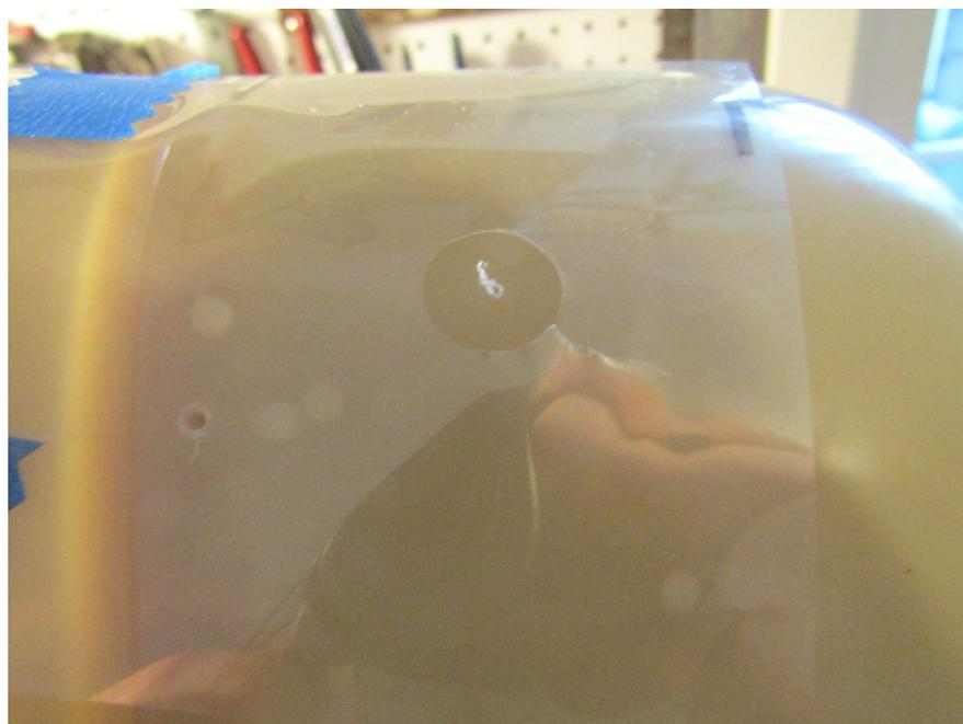
At the drill press, a bit is selected slightly larger than the elbow diameter.
