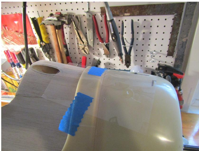
A pilot hole is drilled into the cowl in the center of the hole.
