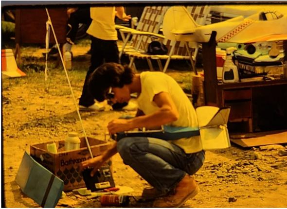
**3-channel MRC radio with slider-tab throttle on left**
