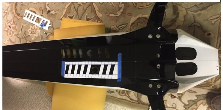
The fuselage has 12 cutouts off the centerline for heat evacuation. They begin under the 3086 cans and extend past the exhaust. They are about  $3\frac{1}{3}$  long by  $\frac{3}{4}$  wide. Hope it's enough.
