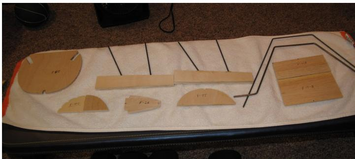
I decided to start with fabricating the wire parts; if I failed, I could bale out before getting in too deep. Alas, I was able to bend the  $\frac{5}{32}$  and  $\frac{1}{8}$  wire just fine, - so no off-ramp there.
