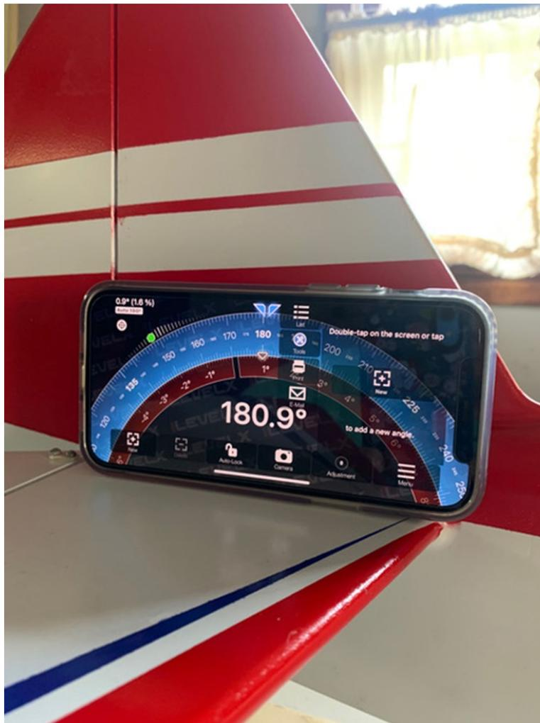
The wing and stab were exactly where they should be at 0.0, and equal on both sides. My meter worked great, but more notable was the quality built GP Sportster 90/120.
