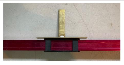
While working on a new plane, I wanted to check the incidence of the wing and tail. According to the plans, they are supposed to be identical at 0.0. The model came to me already glassed and ready for finishing. After setting the fuselage on my worktable, it was showing .9 degrees pitch down. I installed the incident meter. Here are the results:
