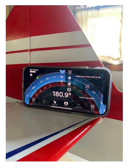
The wing and stab were exactly where they should be at 0.0, and equal on both sides. My meter worked great, but more notable was the quality built GP Sportster 90/120.
