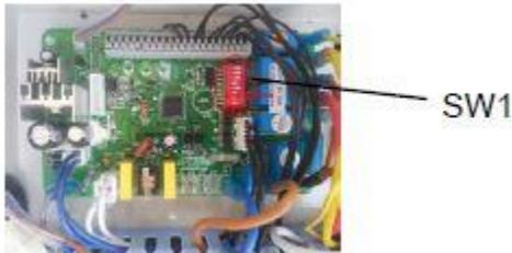
This switch is on the Water System PCB. Unit must be **power cycled** if switch settings are changed.
