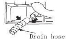
3. Insert the drain stopple into the drain hole on the left side of the indoor unit.
