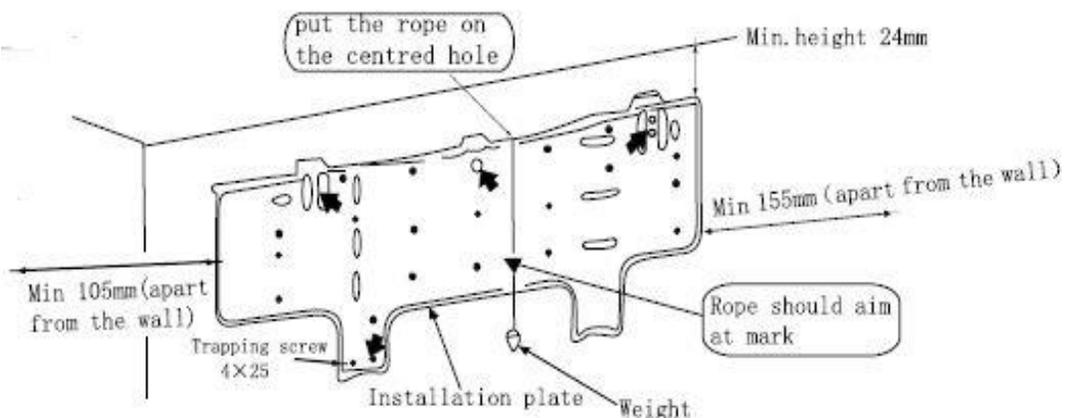
To prevent slight vibration from the installation plate, the holes marked with an arrow must be securely anchored.
