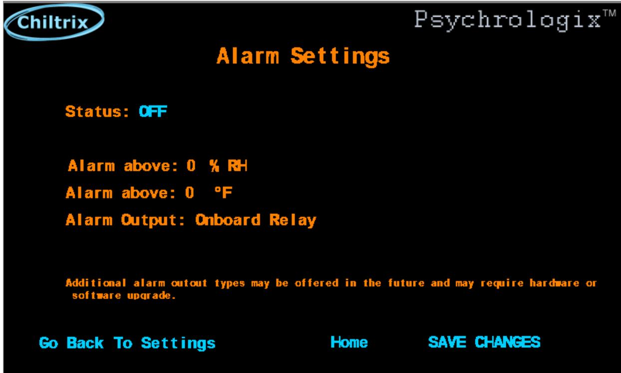
If the alarm status is turned “on”, you must “SAVE CHANGES” to be able to select the relative humidity and temperature values. You can connect a siren, bell, or other device to the system to notify you when a maximum allowable condition has been exceeded. See page 19 for wiring details. Recommended alarm points would be to set T about 5F above the temperature setting you are targeting with your thermostat (or DHC) and set %RH at 65% (or Max H +2-3% of the DHC function) whichever is greater.
