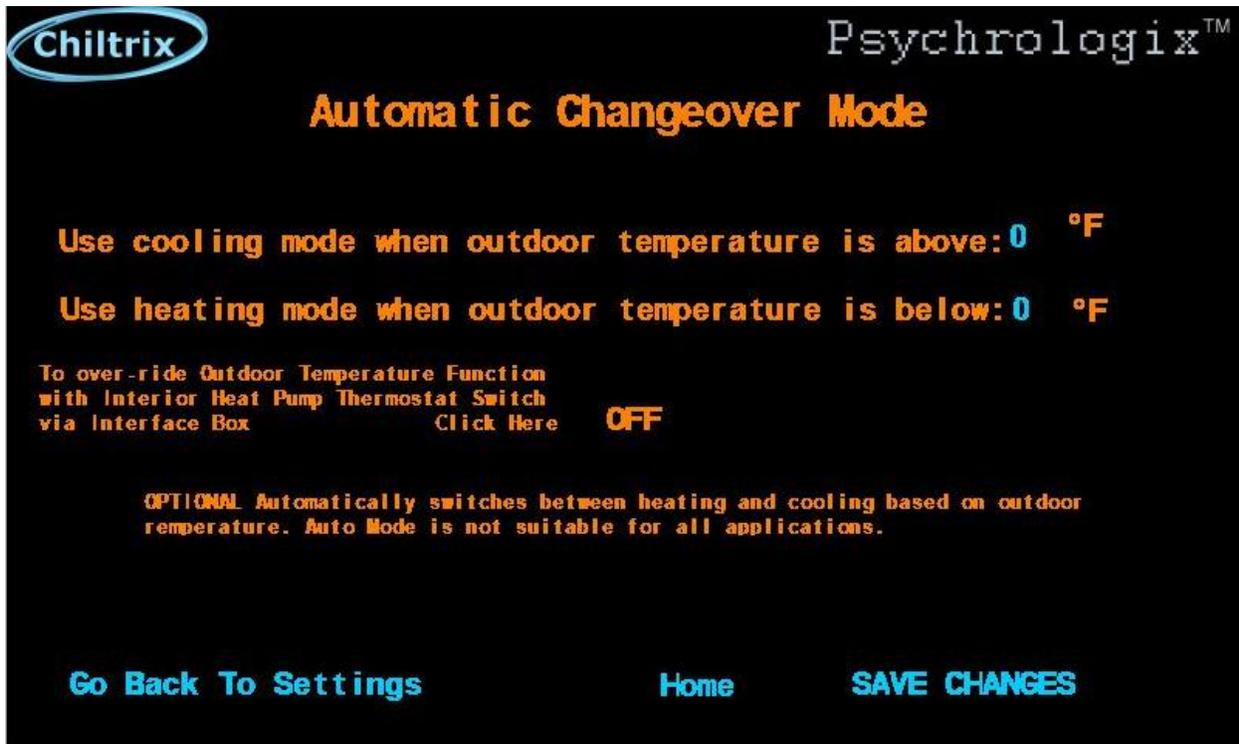
This is an optional feature that can automatically change the system from cooling/heating/standby. Note, this only controls the chiller. The user must still manually select the correct mode of cooling or heating from the indoor unit (FCU etc.) individual controls or other thermostat, as applicable. You may wish to change these settings from time to time as you get used to how it works.
