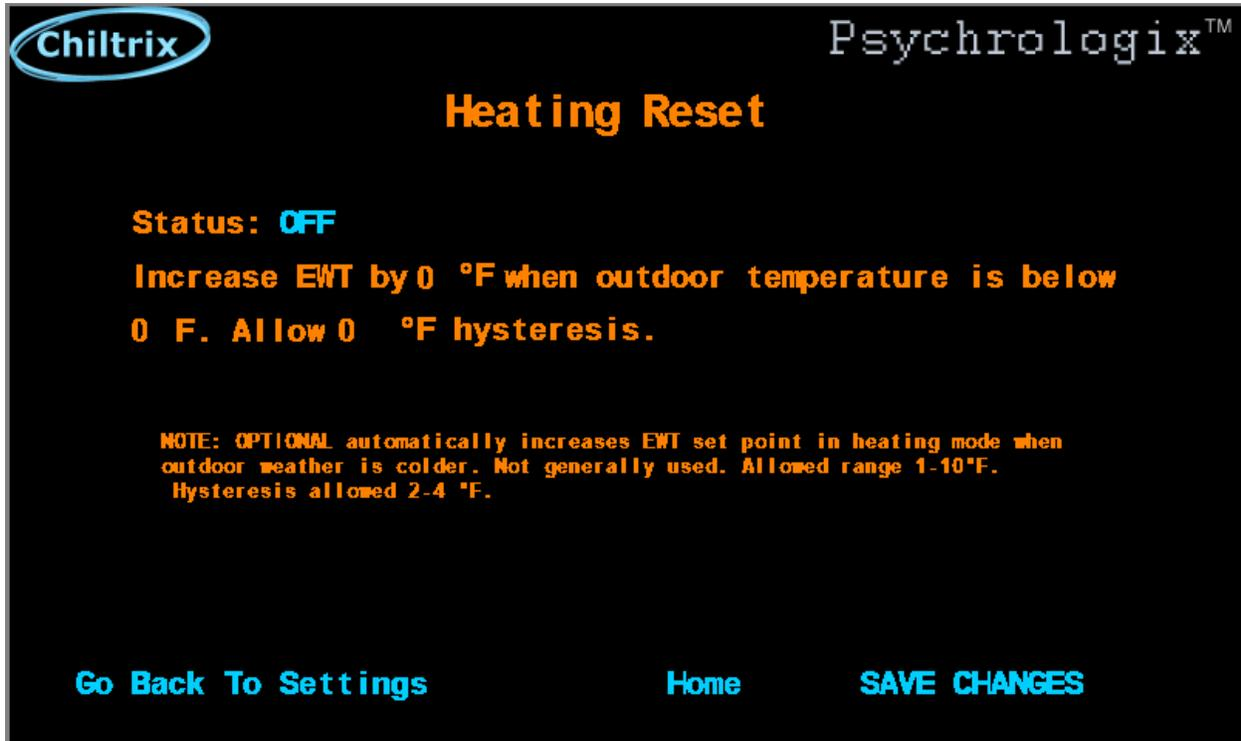
From the Settings screen select Heat Reset if applicable. This is an optional setting used by customers with a radiant heating loop. The idea is that at cold temperatures, a radiant design may not deliver enough BTU/ft<sup>2</sup> when the loop is operating at its normal temperature, to heat the room when heat loss is higher (very cold outside). The Psychrologix controller gives you a single-point reset control.
