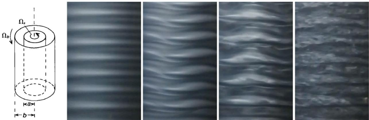
**Figure 1.** (Left) Schematic diagram of the Taylor-Couette apparatus, with differentially rotating cylinders; (Right) sequence of Taylor vortex instabilities, successively breaking continuous symmetries of the flow as the cylinder rotation speed increases from left to right. (Images courtesy of D. Borrero-Echeverry, Willamette University, USA).
