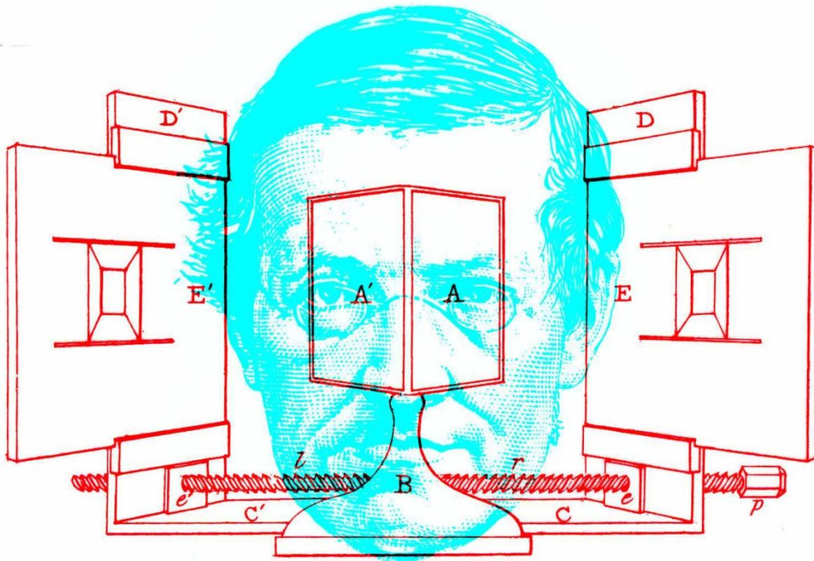
**Figure 2.** *Charles Wheatstone and his stereoscope* by Nicholas Wade. A portrait of Wheatstone together with a diagram of a mirror stereoscope from his original article [2]. The slightly different pictures of a truncated pyramid (E and E', neither of which are symmetrical) are reflected in the mirrors (A and A') to be seen separately by left and right eyes.
