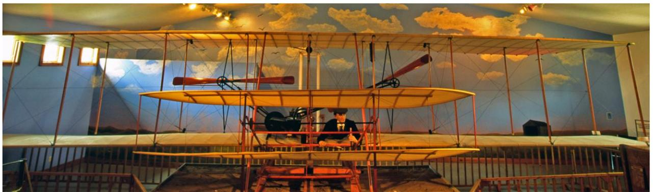
***Wright Flyer*** – This is a full-size replica of the 1903 Wright Flyer. This replica took 10 years to build and was meant to fly. The propellers are hand-carved. The motor is molded and cast into the replica 4-cylinder engine.
