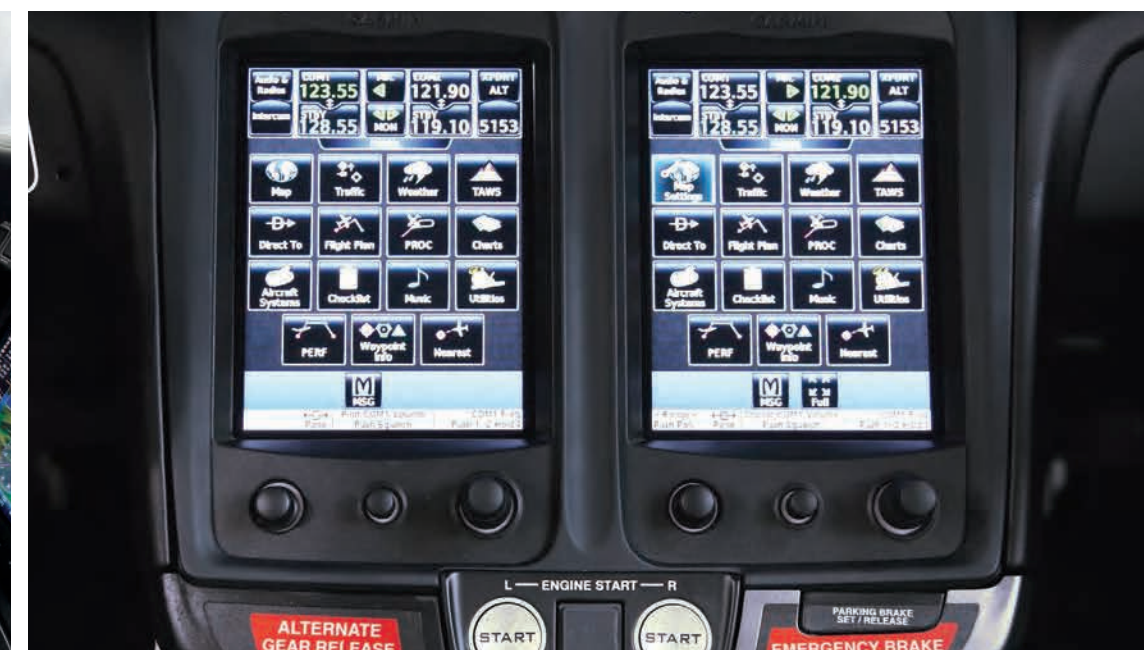
More control at the pilot's fingertips with the dual-glass touchscreen controller on the Garmin G3000 and racecar-inspired start buttons
