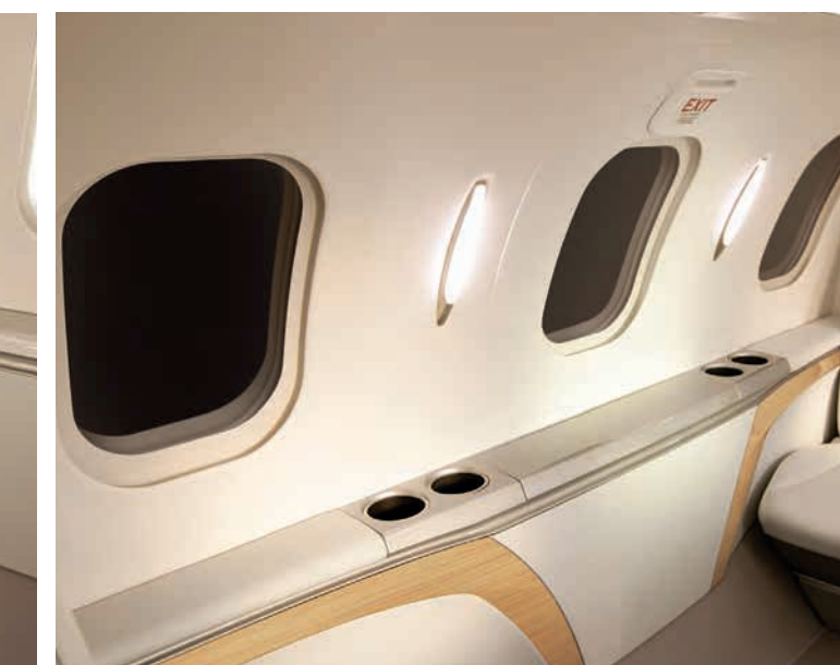
Electronically Dimmable Window (EDW) self-tints upon command
