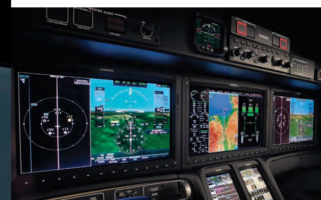
40/60 display format on the Primary Flight Displays enables maximum functional use of display space with easy visual scan for every phase of flight
