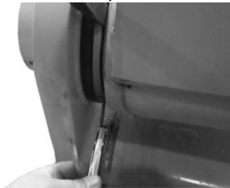
Measuring Bucket Link and Arm End Play
