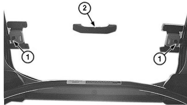
Roof Exit Cover
