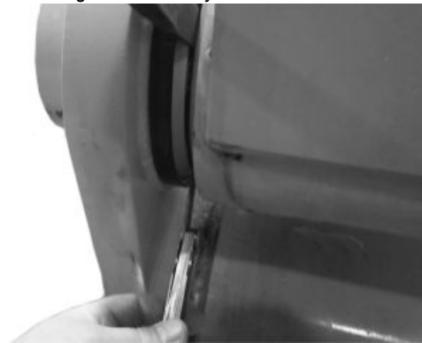
Measuring Bucket Link and Arm End Play
