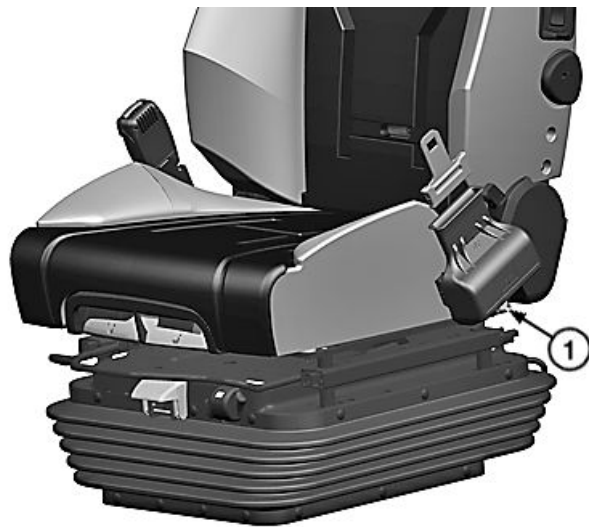
Left Seat Belt-to-Seat Cap Screw (components removed for visibility)
