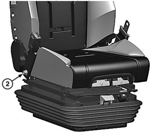
Right Seat Belt Latch-to-Seat Cap Screw (components removed for visibility)
