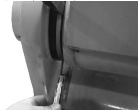
Measuring Bucket Link and Arm End Play
