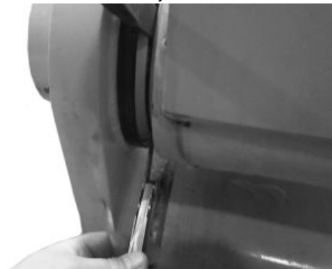
Measuring Bucket Link and Arm End Play
