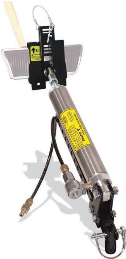
nected between the motorhome and dinghy. The hose runs through a small air reservoir installed under the hood, then runs to a brake actuator installed on the driver's seat floor, which then clamps to the brake pedal. The removable actuator has a quick-disconnect air line. A breakaway system is included.
