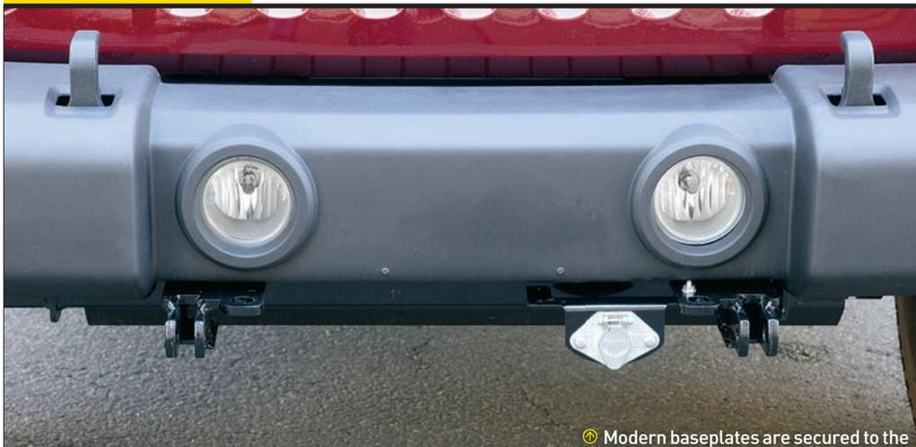
Modern baseplates are secured to the frame of the dinghy vehicle. While some installations are more complicated, the end result is usually a clean appearance.
