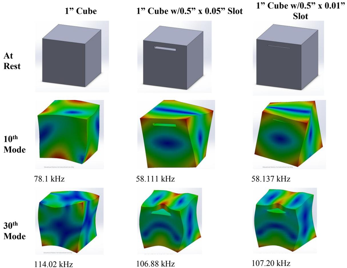
**Figure 2. Simulated vibrations of a 1" cube with slots, illustrating the unique vibration signatures.**
