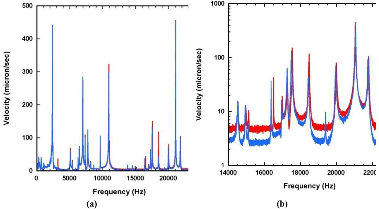
**Figure 11. Effect of a small “defect” on the vibrational spectrum of an extrusion.**
