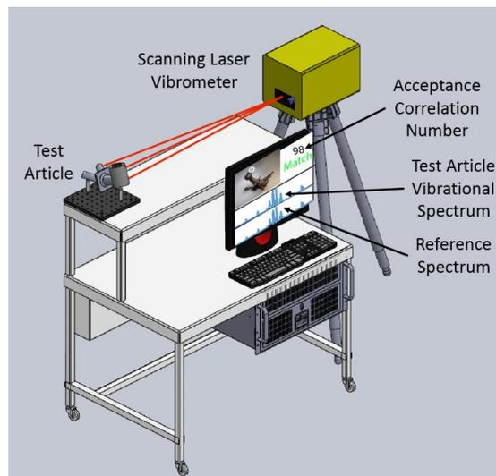
**Figure 1. Conceptual design of the LARS system for component inspection.**
