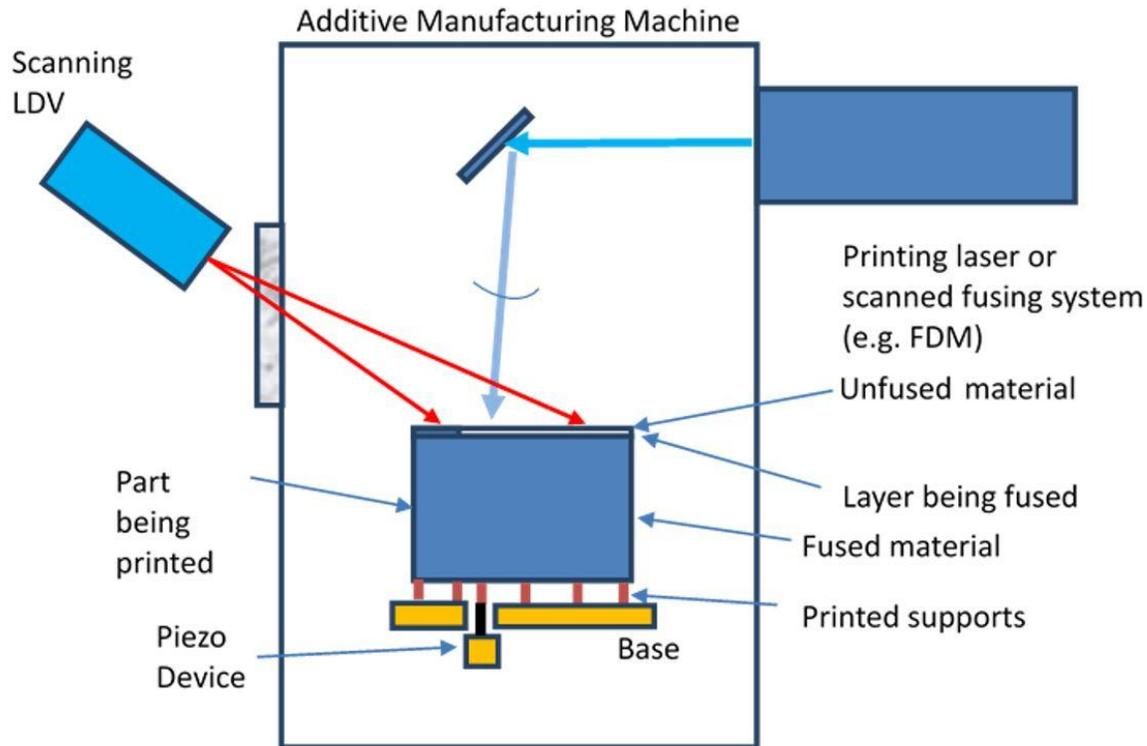
**Figure 9. Conceptual Use of LARS in Additive Manufacturing.**
