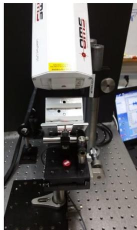
**Figure 5-Component mount showing the foam isolating pads and piezo electric exciter**
