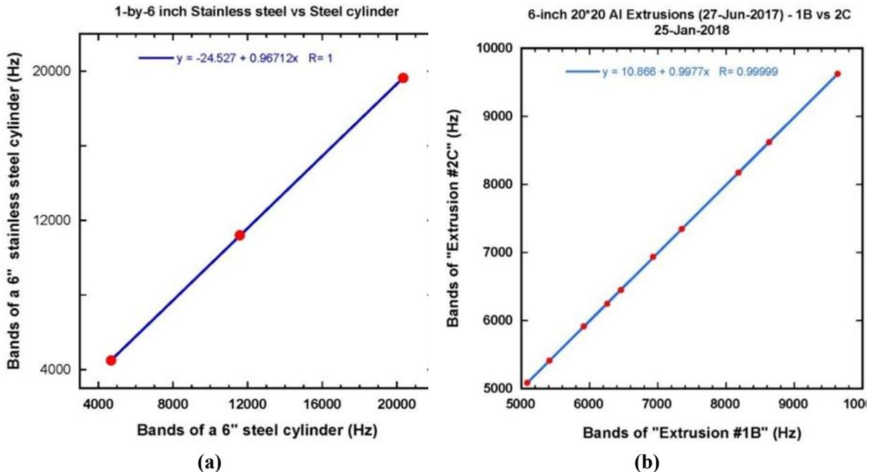
**Figure 10. Comparing vibrational resonances of two identical parts of (a) different materials and (b) two identical ones (a more complex geometry, an extrusion, with more measurable bands in the right panel).**
