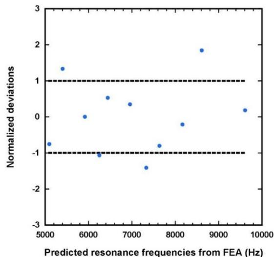
**Figure 12. Measured spectral deviations from those predicted from FEA.**
