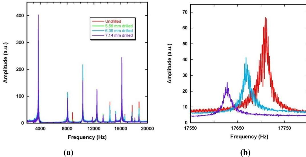
**Figure 8. Vibrational spectra of an AM component with incremental increases in a small drilled hole diameter (left, center, and right as the drilled diameter is increased from 5.56 to 6.63 to 7.14 mm). (a) Entire vibrational spectrum; (b) Enlarged view of the peaks near 17.7 kHz.**
