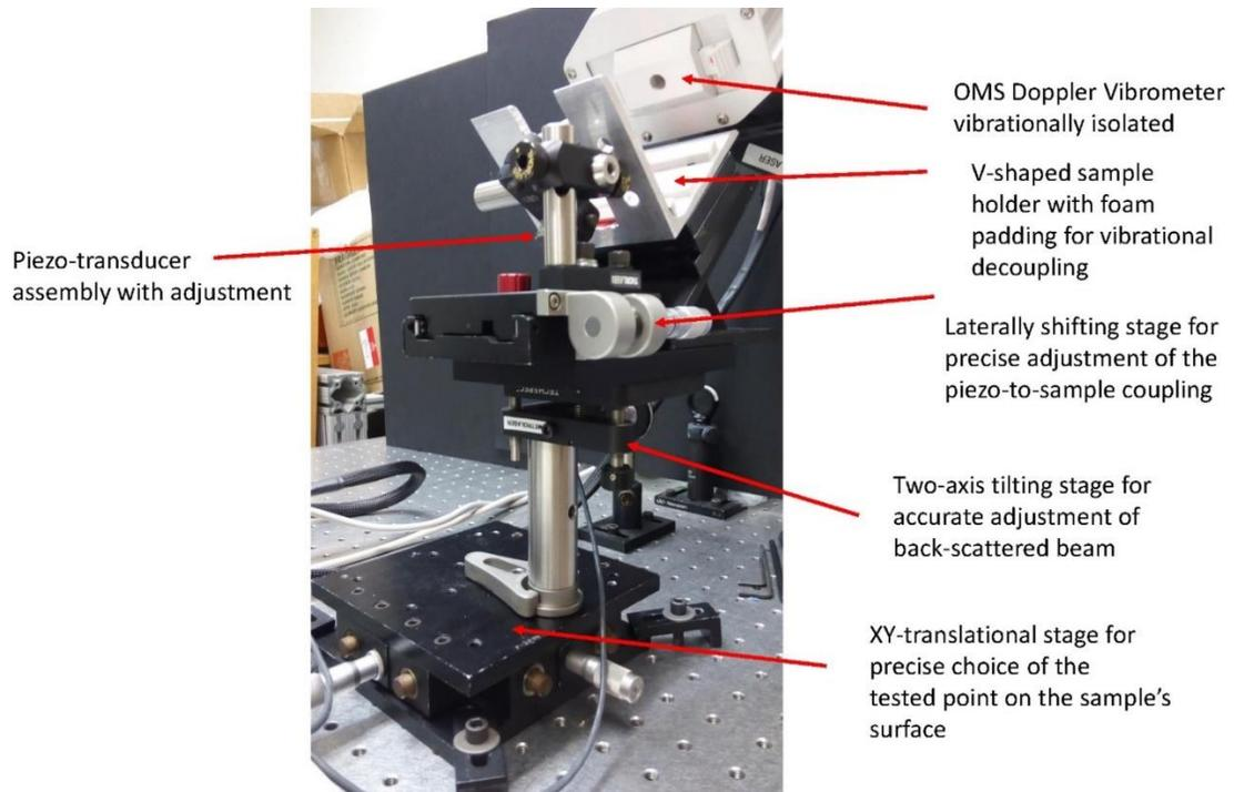
**Figure 4-Explanation of various adjustments for LARS Prototype**
