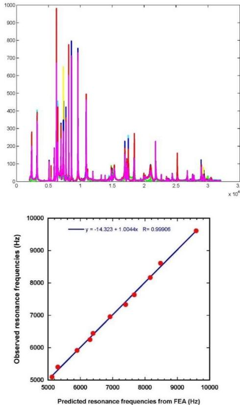
**Figure 13. Comparing vibrational resonances of a part (left panel, several spectra superimposed) with the corresponding bands' positions predicted by FEA.**
