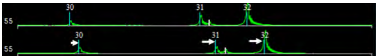
Figure 7 —Resonance Spectra for parts before and after HIP. Change in resonance provides valuable process control feedback.
