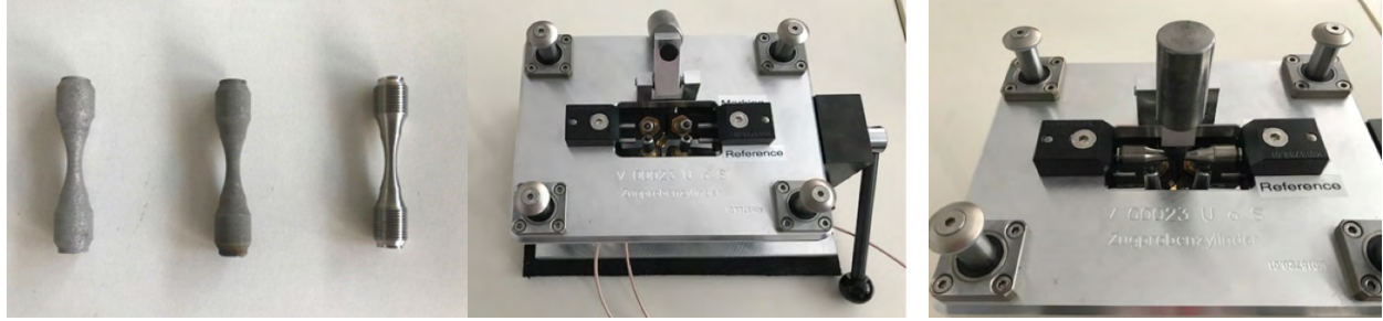
Figure 1 —Photo of AM samples and PCRT fixture
