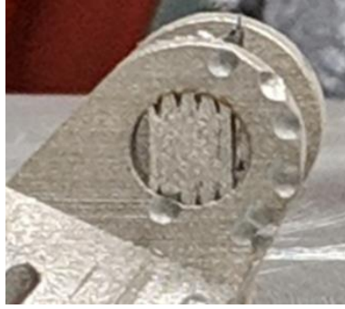
Fig. 68: Damage to parts from BB-gun testing
