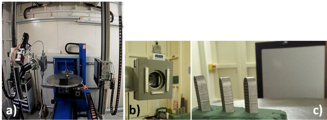
Fig. 6 a XDR Safran system; b XDR Safran source; c XDR Safran detector and photo of the three inspected Co–Cr lattice structures with inner missing struts on the XDR platform
