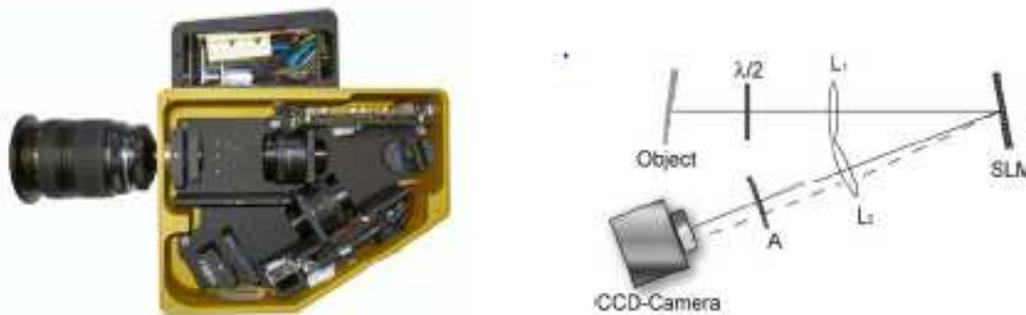
**Figure 2.1. Digital Shearography system** (Huke, Focke, Falldorf, Kopylow, & Bergmann, 2010)
