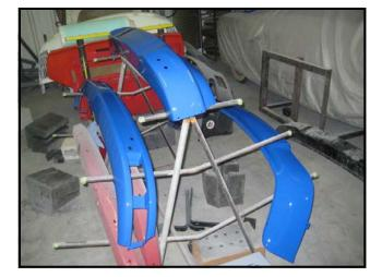
I chose black for a donor car as I was not planning to take it back to a tub and black would be the most palatable color to leave the front trunk and engine bay. The doors were painted off the car and the interior was taped off where the door rubber sits, so the sills and door jams are the same color blue as the exterior but you cannot tell from the photos. I will probably paint the front trunk and the engine bay with black POR-15 to tidy it up but that
