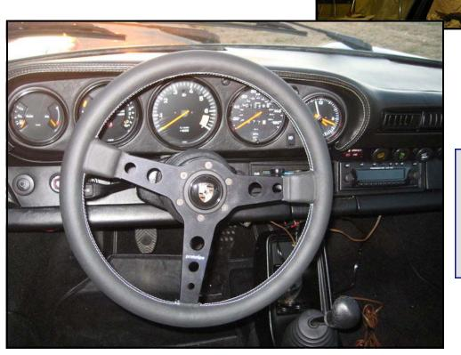
The dashboard has been recovered in OEM type black vinyl. The steering wheel is a Prototipo replica with white stitching so I had a French seam done around the instrument binnacle in the white also.
