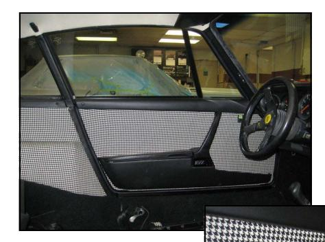
Sometimes it's the little details...note the "911" script on the door release. And why the tape on the power window switches? To protect them during reassembly, of course. A sign of care and professionalism...
