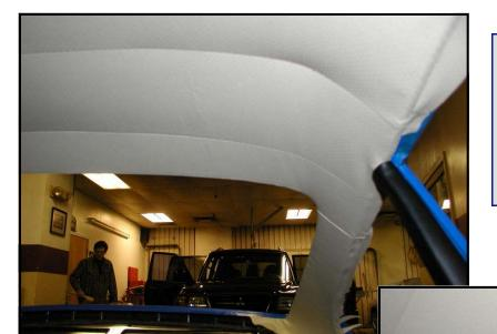
And attention now turns to the interior. Headliners typically show some wear, and of course are very visible. While a headliner can be replaced without painting the car, while it is disassembled for paint it is the best opportunity. Replacement headliners are readily available, and are carefully trimmed to fit.
