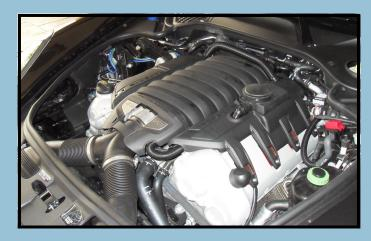
A 4.8 liter, 400hp V8 powers the Panamera S. With a dry sump oiling system, 4 valves per cylinder and VarioCam Plus valve timing, the lineage of this engine is clear.
