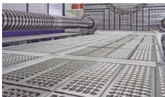
Equipped with a large-area safety pedal to provide safety protection for the mold clamping area (9000kN and above).
