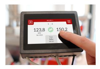
4.3" capacitive color touchscreen controller with modern functionalities for injection moulding, blow moulding and extrusion processes.
