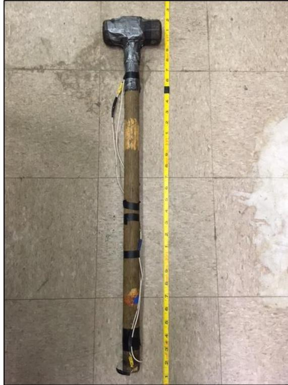
Figure 2.4. This is the hammer. A user stands atop the shear-plate and manually applies a force to the shear-plate by striking the left/right side of the plate. This action generates and transmits a shear-impulse into the earth. The weight of the hammer is ~4.22 kg.
