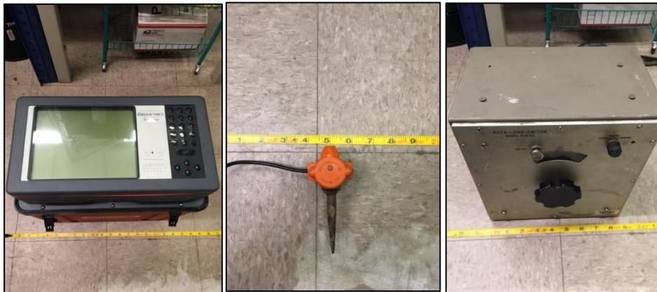
Figure 2.10. I use the Geometrics R-24 Strataview (left) to set the sampling rate, file structure, and record all seismic data for this study (Figure 2.12). A single Mark Products, 30-Hz, geophone (middle). As the geophone is situated for this image, it detects motion into and out of the page. The rota-long-switch (right) is connected to both the 48-channel take-out cable and Geometrics R-24 Strataview. The rota-long-switch allows for successive reconfiguration of channels for each shotpoint
