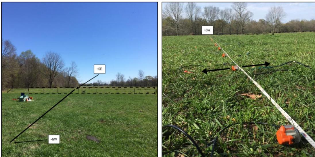
Figure 2.13. The inline survey ground perspective (left) from position 1 (Figure 2.12). The solid black line represents the position and orientation of the inline survey. The dashed box at the middle partially encloses a topographic high immediately before the topographic low area (Figure 2.12). Position 2 (Figure 2.12) captures part of the crossline survey (right). The black arrows on either side of the geophone indicate the primary ground motion that is measured during data acquisition.
