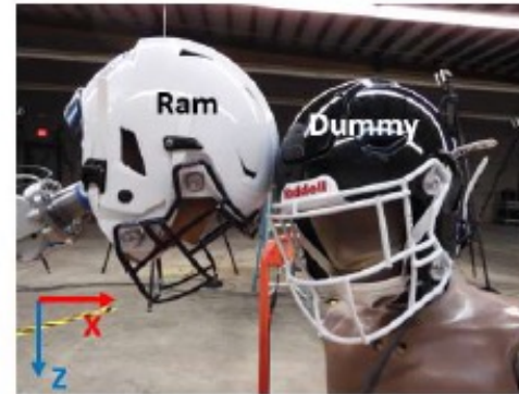
Test Condition #1 (5cm eccentric) Ram Front to Dummy Front Oblique
