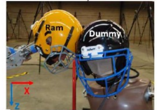
Test Condition #2 (10 cm eccentric) Ram Front to Dummy Rear Eccentric
