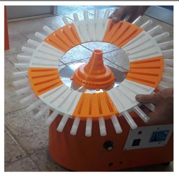
→ The HUB and the OUTER RING must be attached before use. They can also be REMOVED FOR CLEANING
