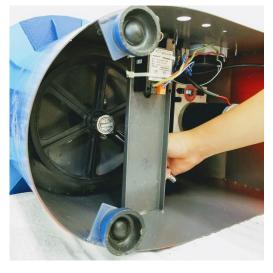
LOOSEN the nuts that hold the motor and the belt, then slide the motor forward to loosen the belt. Remove the belt, but NOT the motor.
