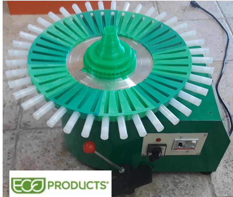
**NOTE: GREEN MACHINE ONLY - Set Sealer on 5 (empty straws) and 7 (full straws) and hold the arm down for 10 SECONDS - to prevent pinhole leaks. EXPERIMENT.**
