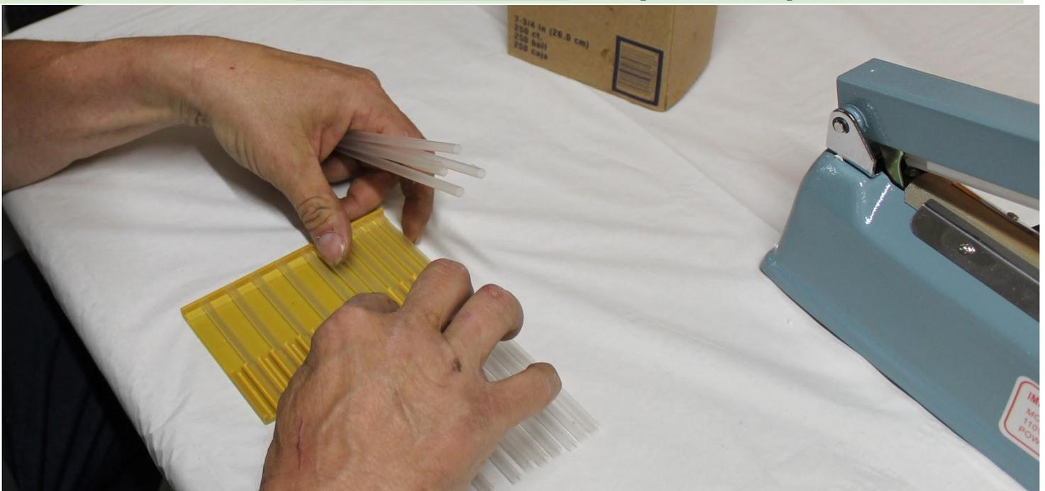
→ Seal Straws on one end, using the impulse sealer included with the machine.
