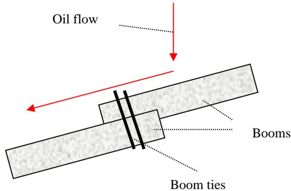
When deploying oil booms across a river, stream etc, it should be set up so that it forms a tick, as shown below. This makes removal of the oil from the water much easier.
