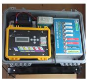
Enables full manual control and override of ADDCO PTS-2000 portable traffic signals for applications such as a drawbridge operation within a work zone that includes portable traffic signals, fire station control for direct preemption activation, and many more custom uses.
