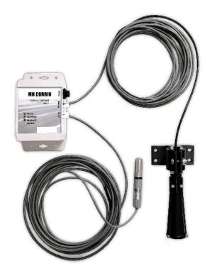
The SurfaceScan is a vehicle mounted mobile weather sensor. The sensor monitors road surface temperature, air temperature, relative humidity and dewpoint, as well as displays live readings using a dash mounted graphical display. The SurfaceScan can be used to detect freezing temperatures on the pavement to determine where frost or black ice may form if precipitation occurs.
