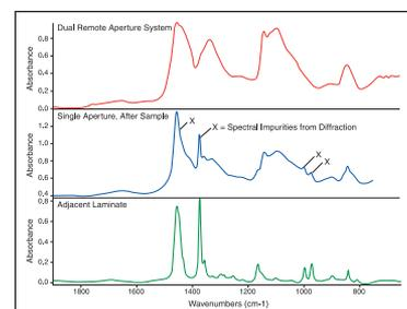
Figure 19: Upper spectrum collected on Continuum microscope with Reflex aperture. Middle spectrum collected from another vendor's IR microscope system with single aperture showing interfering data from the surrounding sample area. Lower spectrum collected from surrounding sample medium
