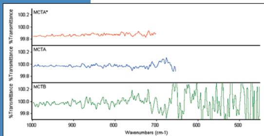
Figure 16: Spectral range vs. spectral noise for several MCT detectors
