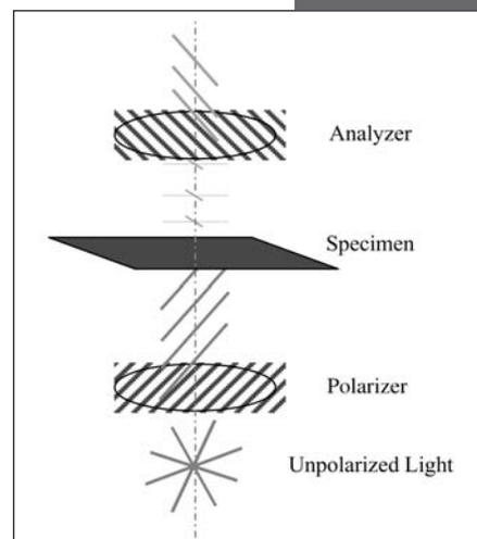
Figure 8: Polarized light ray trace
