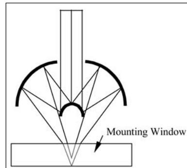
Figure 24: Spherical aberration causes a blurred image if not compressed
