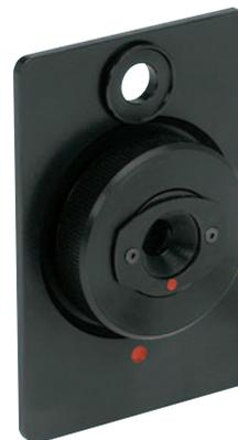
Figure 23: Microcompression cell
