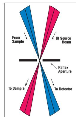
Figure 20: The automated Reflex aperture provides dual masking with a single aperture for the highest spectral quality and maximum ease-of-use
