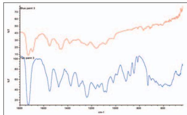
Figure 18: Automotive paint samples collected on Continuum with MCTB
