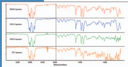
Figure 17: Performance advantages of the 50-micron detector with small sample sizes
