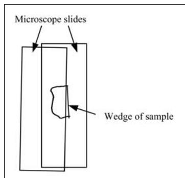
Figure 22: Simple microtome using glass slides
