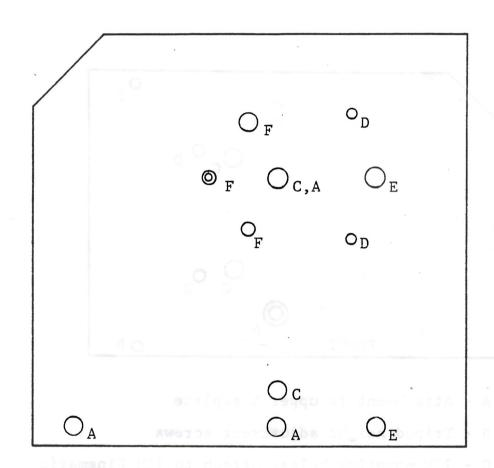
Install plate into spectrometer compartment as described, then mount CIRCLE onto mating plate through (D) holes
