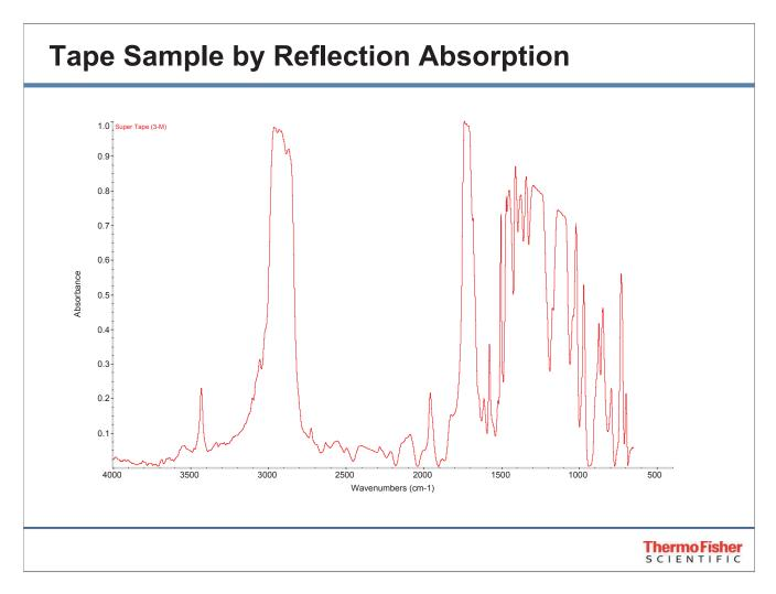
Here a reflection absorption spectrum is nearly identical to a transmission spectrum. In many ways, this type of analysis can be thought of as a double transmission analysis because the infrared energy will pass through the sample twice. This often leads to totally absorbing bands if the sample is too thick so care must be taken in preparing the sample for analysis.
