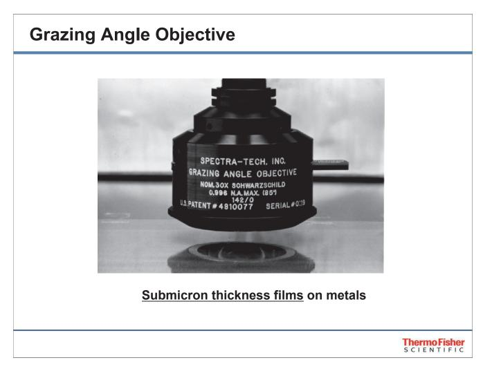
The grazing angle objective has a specific optical path defined by an aperture that only allows the more extreme angles to pass through to the sample surface. This creates a low energy situation. The loss of energy will be manifested in the sensitivity of the experiment. It is not uncommon for the number of scans required to clean up the noise to run into the thousands.
