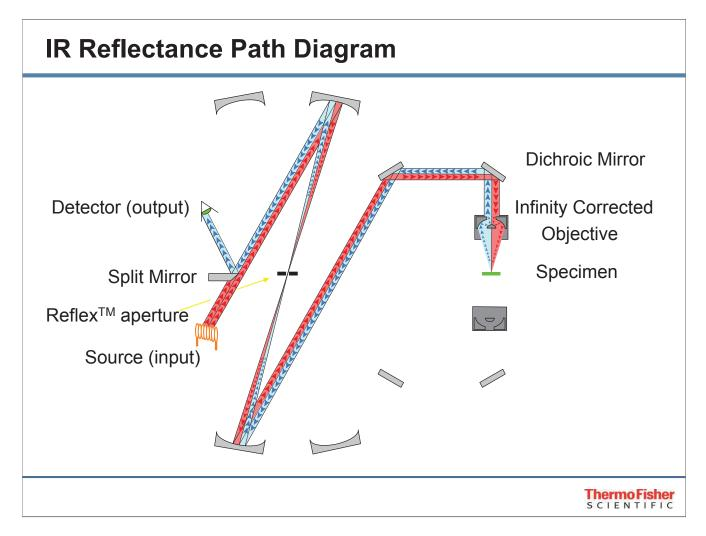
Reflection alignment is much easier than transmission alignment. The condenser should be safely stowed by bringing it to its lowest setting. Since energy will be transmitted and collected from the objective, the expected performance is worse than transmission performance. Note the split mirror used to direct the reflected energy to the detector. For transmission analysis this mirror is rotated out of the beam path.
