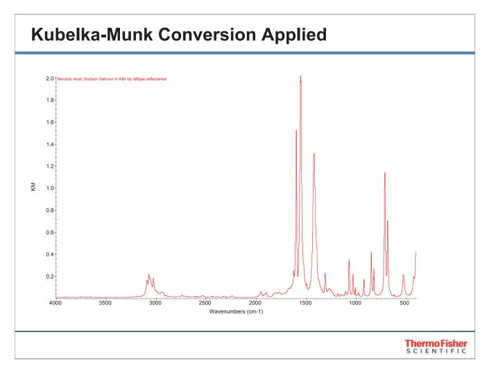
Select Kubelka-Munk in the Other Conversions dialog box to convert %reflectance spectra collected using the diffuse reflection (DR) technique to Kubelka-Munk units. These units are similar to absorbance units. As a result, the Kubelka-Munk format is useful for visually comparing diffuse reflectance spectra against absorbance spectra in commercially available libraries.
