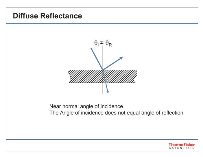
Diffuse reflectance is typically utilized as an analysis method for powders or granular samples. Using this method, some energy scatters off of the sample surface at angles other than the incident angle.
