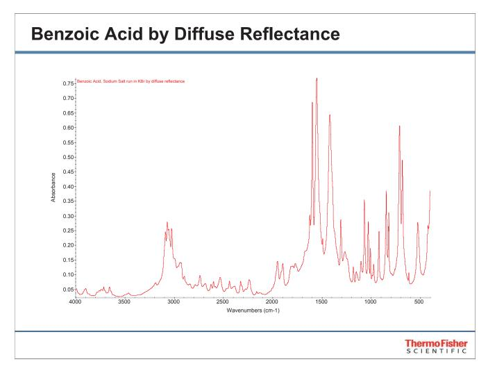
This is a spectrum of Benzoic Acid in KBr taken by diffuse reflectance. In many cases, the concentration of samples analyzed using the diffuse reflection technique do not vary linearly with log (1/R) (which is the equivalent of absorbance for reflection measurements) this is due to pathlength variation. The Kubelka-Munk scale was developed to provide a more linear relationship with respect to concentration.
