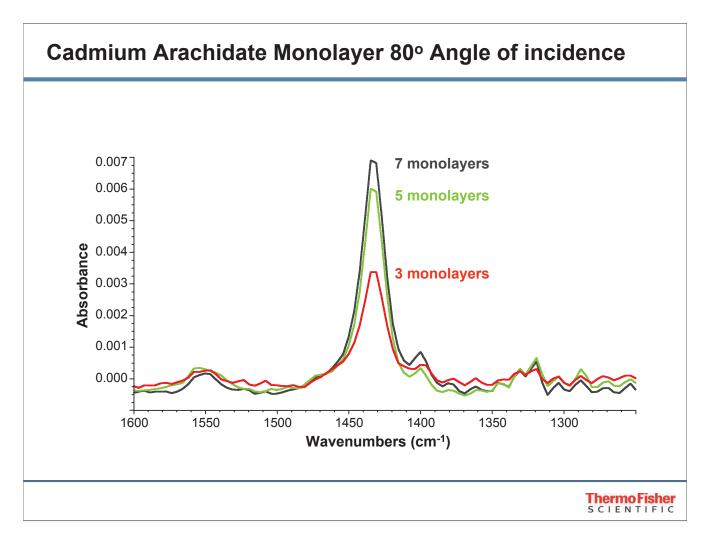
These are spectra of samples of Cadmium Arachidate monolayers on a gold substrate. Data is shown for samples with 3, 5, and 7 monolayers deposited.
