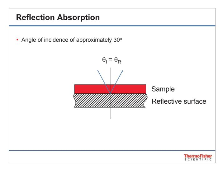
In this experiment the light passes through the coating material to the reflective surface and back out. In order for this experiment to provide clean data the surface of the coating as well as the surface of the underlying material need to be smooth. Any rough surface will scatter the infrared energy and will cause inconsistencies in the measurements.
