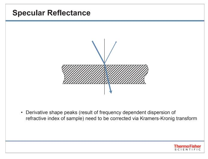
Specular reflectance occurs when light energy is reflected off the surface of the sample at an angle near normal. The reflected energy is then collected at the same angle. The interaction that occurs at the reflection point is what is being measured.
