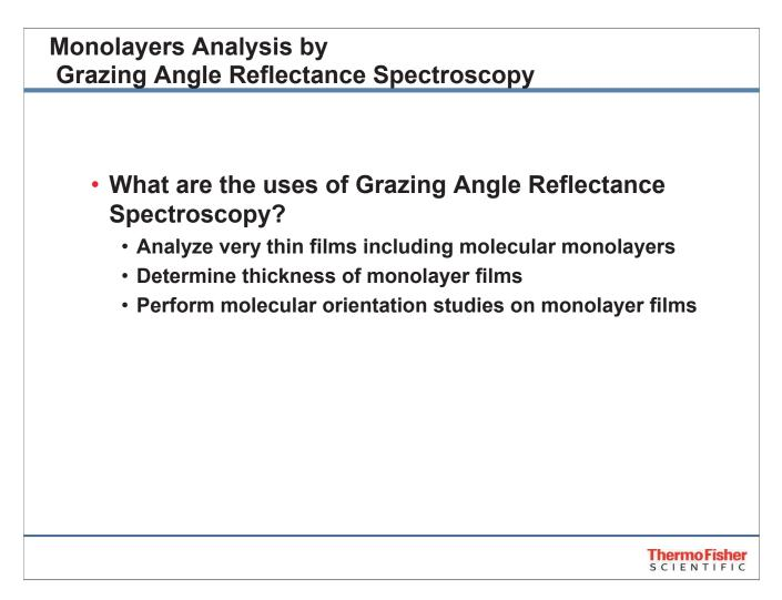
Grazing angle measurements are commonly used to measure ultra-thin films from 1  $\mu$ m to 10 Å. Even monolayer films can be analyzed with grazing angle when they are on reflective metal surfaces. Grazing angle analysis can be used to measure thickness and study molecular orientation.
