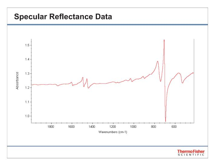
The combination of interactions combined with the shift in energy due to the non-ideal background causes the appearance of the acquired data to be non-conventional. Don't let the appearance fool you. This is perfectly good data. Quantitatively the goal is ease and reproducibility of which both are obtained. Any quantitative analysis should use this form of the data along with the PLS algorithm provided in the TQ Analyst software.
