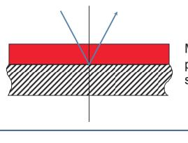
Multiple reflection points can cause sinusoidal wave
