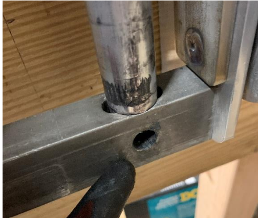
Figure 2 - Spring Pin Removed
