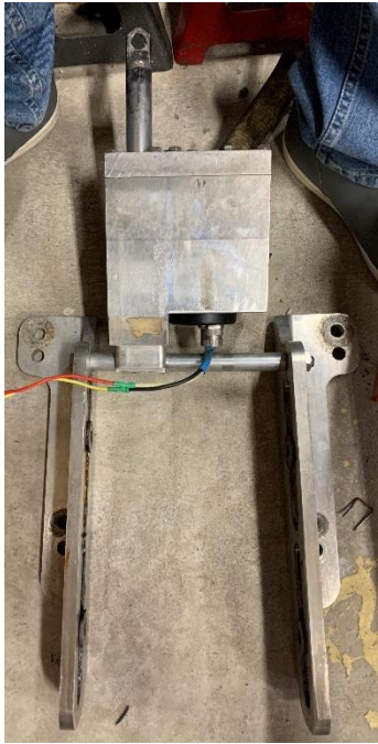
Figure 4 - Actuator and Engine Brackets set aside
