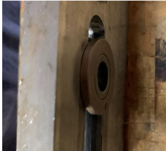
Figure 8 - Ensure Thick Washer is on the inboard side
