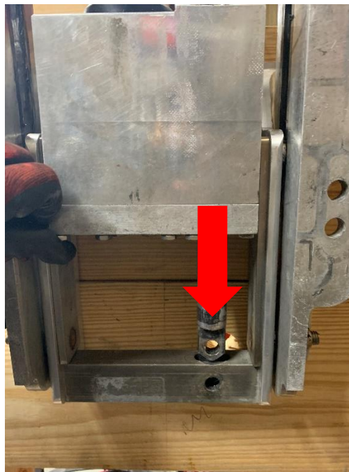
Figure 12 - Insert Actuator Rod into Pocket
