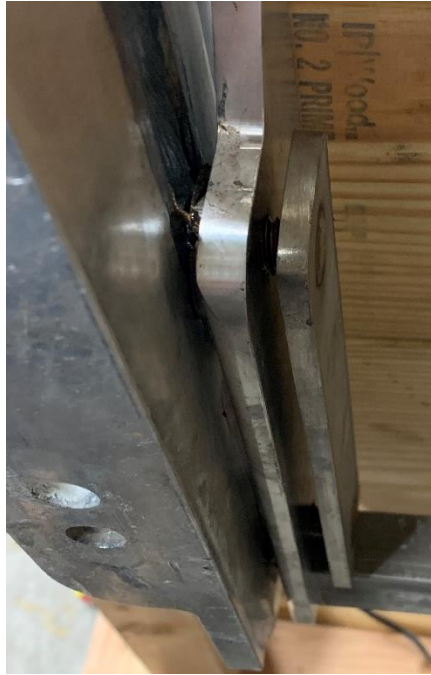
Figure 9 - Reinforcement Plate Inserted into Transom Bracket
