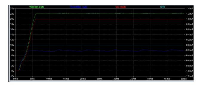
As shown, our load output voltage stabilizes at around 20V with a ripple of 20mV. Similarly, our load current is zero since it is an open circuit.
