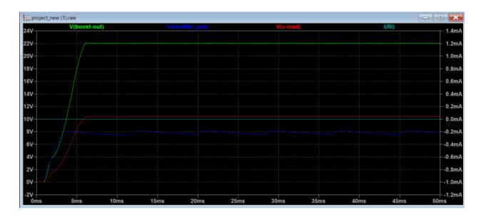
We can see that the load output voltage stabilizes around 10V, with a ripple of 20mV. Similarly, we see that the load current is zero, since it is an open circuit.
