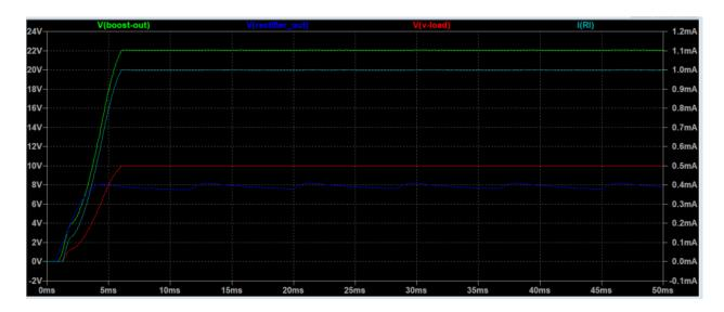
We can see that the load output voltage (shown in red) stabilizes at 10V with 20mV of ripple. Similarly, the output current (shown in teal) is capped at 1mA.
