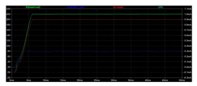
We can see that our load output voltage stabilizes around 20V with a ripple of 20mV. Similarly, the load current is capped at 1mA.
