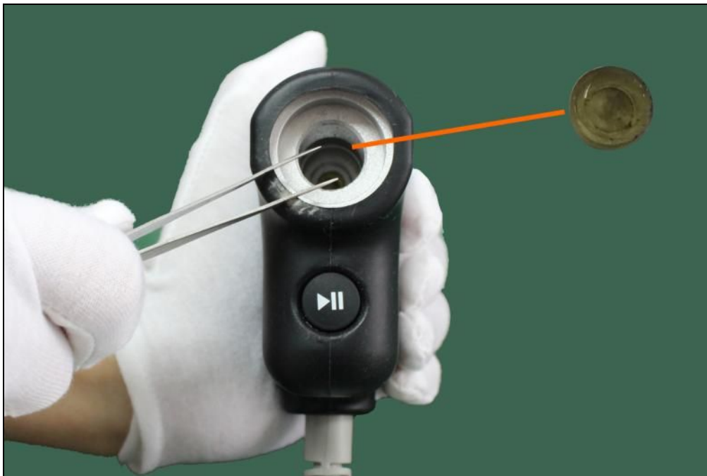
Step 2: Take out of the old spacer with a tweezers.
