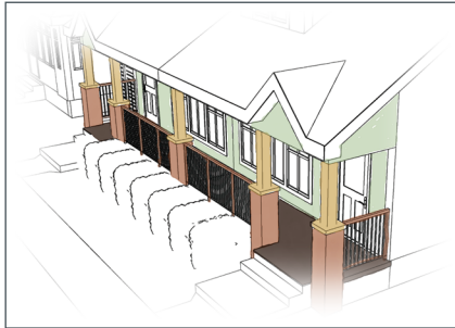
Full width verandah
