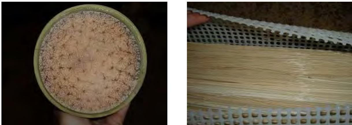
**Figure 3.18 Membrane A module (end view and fiber bundle)**
