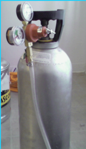
High Pressure Nitrogen and Beer Gas Cylinders
