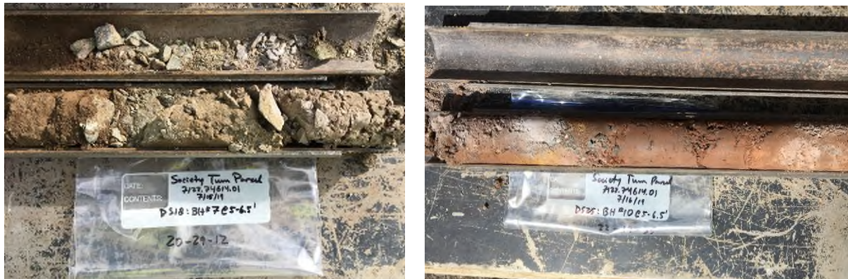
Photo 4 (left) shows the native soils from BH#7 at 5-6.5 feet and Photo 5 (right) shows the soil from BH#10 at 5-6.5 feet. Soils range from light brown to red-brown and are generally silty/clayey sand and gravel.
