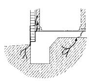
Figure 4.18. Monolithic slab tile floor (arrows indicate possible termite entry points).
