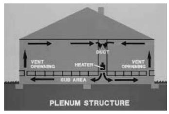
Figure 5.1. Plenum houses use the area under the subfloor as a giant heating/cooling air chamber. Because of this, use of conventional liquid termiticide is not recommended.
