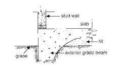
Figure 4.3. Monolithic slab construction.
