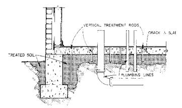
Figure 4.11. Treatment under concrete with vertical drilling at joints, cracks and openings, and around plumbing.
