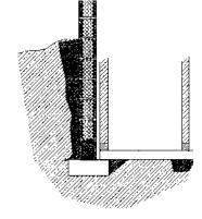
Figure 4.22. Completed treatment of basement construction (dark shading indicates areas treated).
