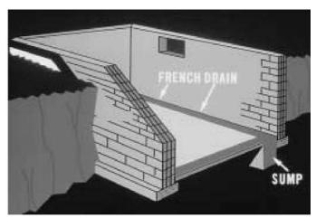
Figure 5.4. A French drain is a below grade drainage system that is level with or beneath the basement floor and usually runs around its perimeter. When water gets into the basement it goes through the French drain and runs into a sump or sometimes outdoors.
