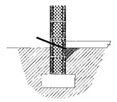
Figure 4.12. Short rodding (dark shading shows area treated).
