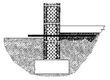
Figure 4.13. Long rodding (dark shading shows area treated).
