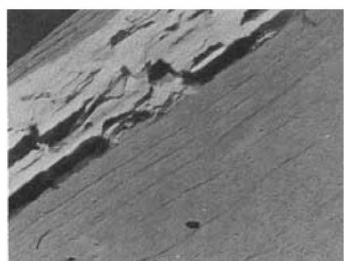
Figure 6.14 Old house borer damage with oval exit holes and powder-filled galleries in interior of wood.
