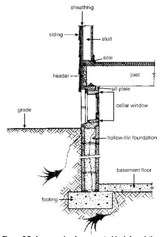
Figure 5.7. An example of a concrete block foundation with basement window. Avenues of termite access are indicated by the heavy arrows in the soil (NPMA).
