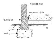
Figure 4.2. Floating slab construction.
