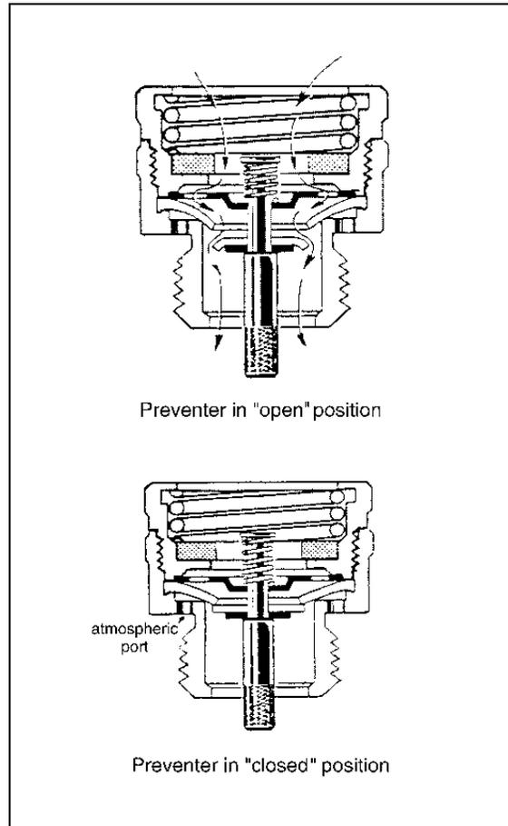
**Figure 3.8.** Backflow preventer in open and closed positions.
