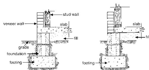
Figure 4.4. Suspended slab construction.
