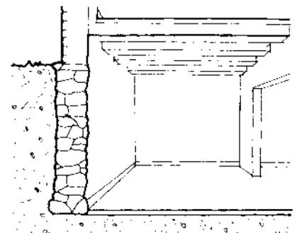
Figure 4.6. Basement construction.
