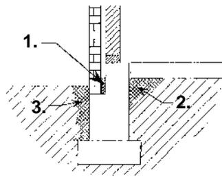
**Figure 4.17. Completed treatment of poured foundation—brick veneer showing treatment of 1. the voids in the brick veneer, 2. the subslab soil area along the expansion joint, and 3. the outside perimeter of the building.**
