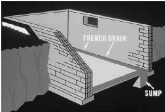
**Figure 5.4.** A French drain is a below grade drainage system that is level with or beneath the basement floor and usually runs around its perimeter. When water gets into the basement it goes through the French drain and runs into a sump or sometimes outdoors.
