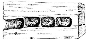
Figure 4-8. Carpenter bee tunnel and larvae. Carpenter bees prefer to tunnel in seasoned wood and reuse these galleries year after year.
