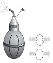
dusters consist of a Figure 1-5. Bulb duster. This closed rubber cylin- sprayer is used to apply pesticide der made rigid by an dusts to cracks, crevices and other internal spring, with a
