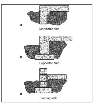
Figure 2-13. Three common types of slab foundations. A monolithic slab (a) is a single, solid unit of concrete that forms both the slab and foundation walls. A supported slab (b) partially or fully rests on the concrete foundation walls. A floating slab (c) is a sheet of concrete poured directly on soil that butts up to separate slab foundation walls.
