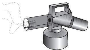
Figure 1-4. Thermal fog generator. This sprayer uses heat to vaporize oil in oil-based pesticides and makes an aerosol fog that can be used to fill enclosed spaces.
