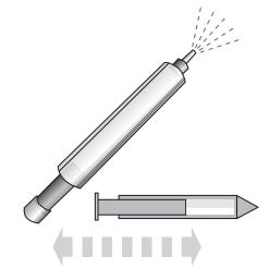
Figure 1-6. Plunger duster. This sprayer is used to apply larger amounts of dust to enclosed spaces.
