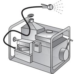
Figure 1-2. Power sprayer. This sprayer uses an electric or gasoline engine to pump large amounts of pesticide from a tank at various pressures. Low pressure is recommended for soil applications around structures.
